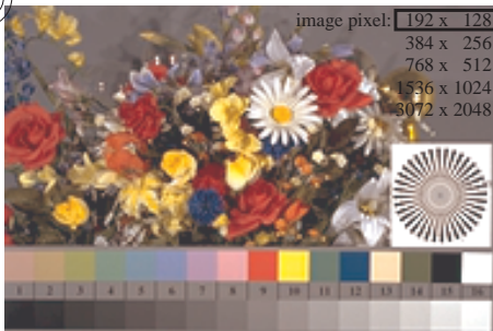
Picture B1: Flower motif, 14 CIE-test colours and 16 grey steps (sf); PS operators settransfer , 4 colorimage
