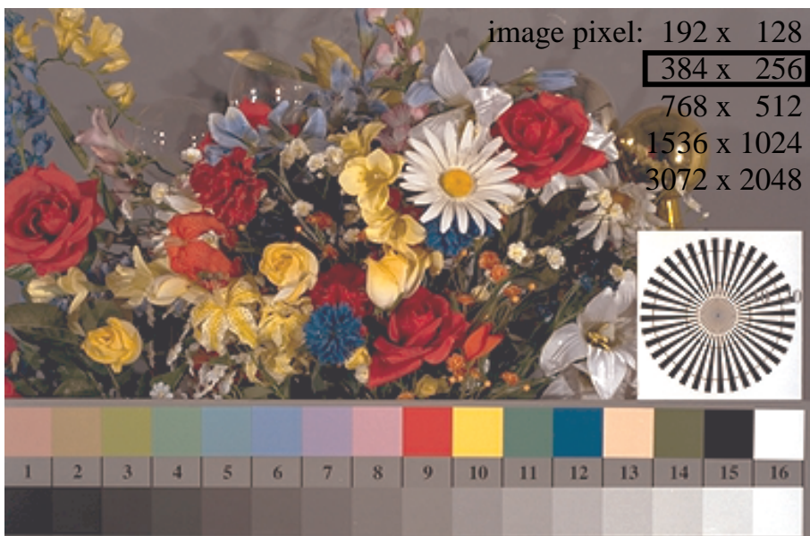
Picture D1: Flower motif, 14 CIE-test colours and 16 grey steps (nf); PS operators settransfer , 4 colorimage
