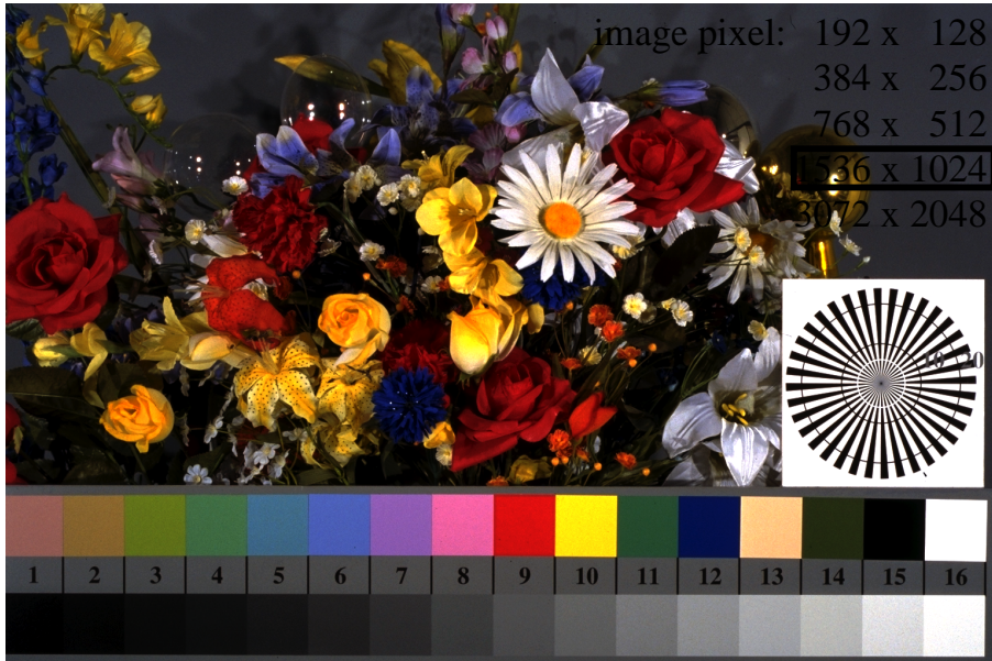
Picture B1: Flower motif, 14 CIE-test colours and 16 grey steps (sf); PS operators settransfer , 3 colorimage
