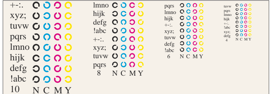
Picture B5: Script and Landolt-rings N, M, C and Y; Use of PS operator cmy0*/000n* setcmykcolor
