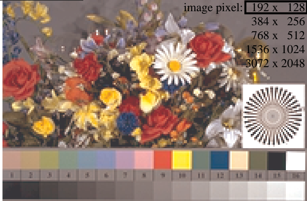
Picture B1: Flower motif, 14 CIE-test colours and 2 + 16 grey steps (sf); PS operators settransfer , 4 colorimage
