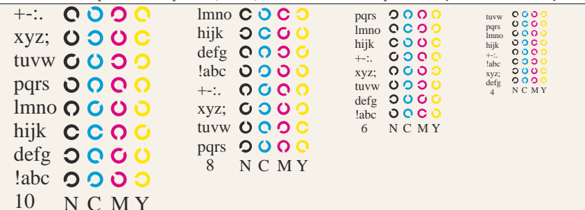
Picture B5: Script and Landolt-rings N, M, C and Y; Use of PS operator cmy0*/000n*setcmycolor
