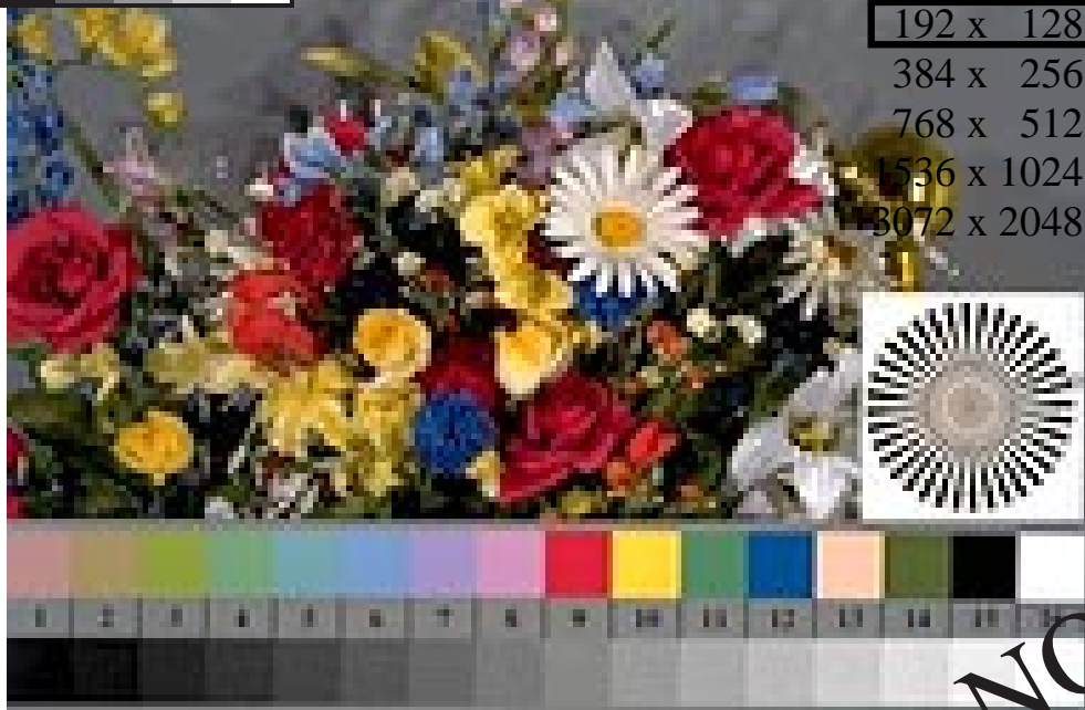
Picture D1: Flower motif, 14 CIE-test colours acc. to CIE publ. 13.3, and 2 + 16 grey steps; negative film (nf)
