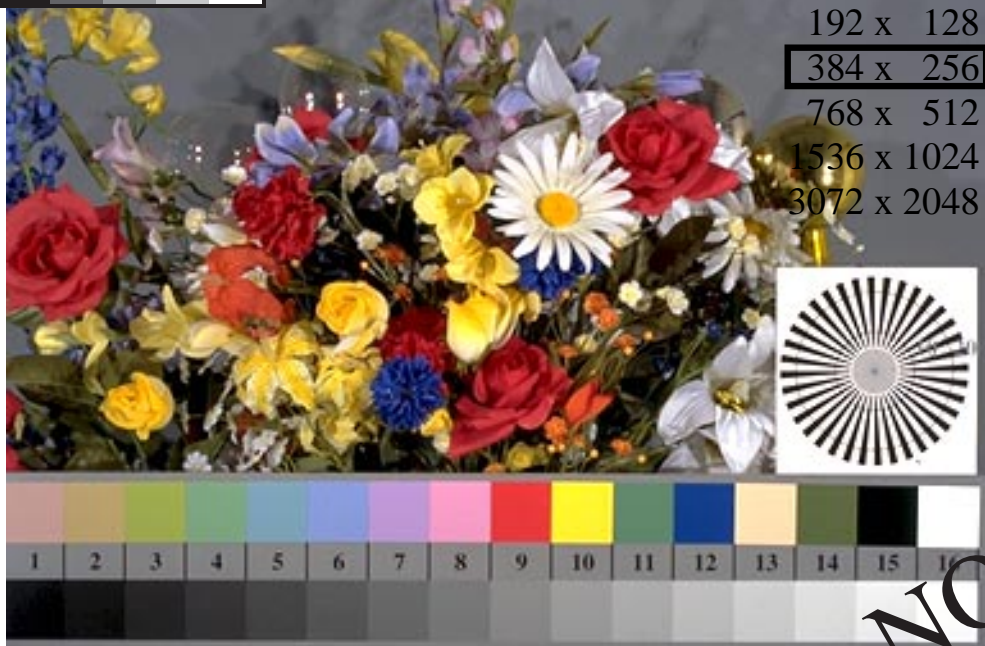
Picture B1: Flower motif, 14 CIE-test colours acc. to CIE publ. 13.3, and 2 + 16 grey steps; slide film (sf)
