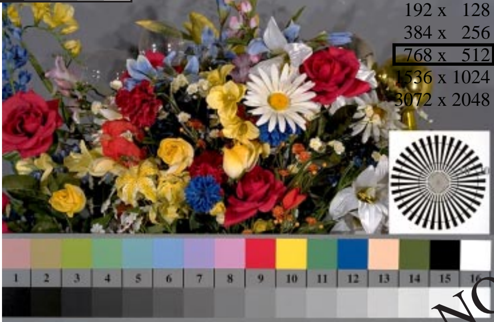
Picture D1: Flower motif, 14 CIE-test colours acc. to CIE publ. 13.3, and 2 + 16 grey steps; negative film (nf)
