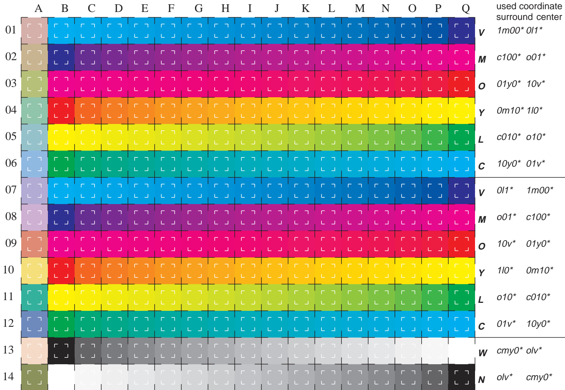
16 equidistant CIELAB steps in cmy0^* and olv^* for colour series C-V, V-M, M-O, O-Y, Y-L, L-C, N-W, W-N and 14 CIE-test colours (left)
