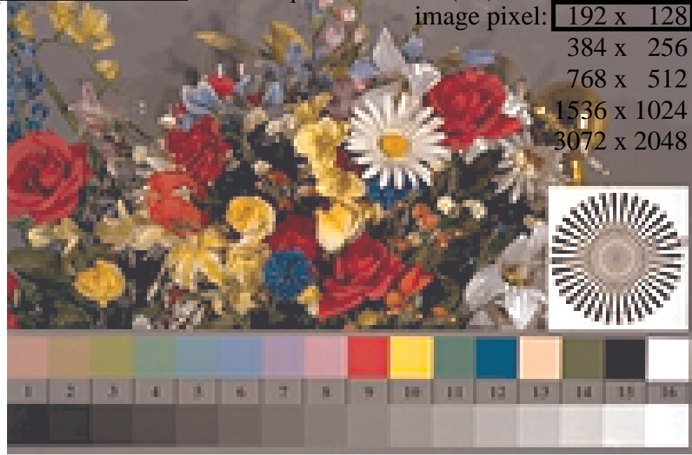
XE730-3, Picture D1: Flower motif, 14 CIE-test colours and 2 + 16 grey steps (nf); PS operators settransfer , 4 colorimage
