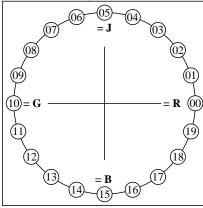
There are four elementary hues on each page: Red R, Yellow J (=french Jaune), Green G, and Blue B. Input data 1 0 0 should produce Red R. Input data 0 1 0 should produce Green G. Input data 0 0 1 should produce Blue B. Input data 1 1 0 should produce Yellow J. Four hue steps are between: Red R and Yellow J, Yellow J and Green G, Green G and Blue B, and Blue B and Red R. This test uses a hue circle with 20 hues All 20 hues should be distinguishable. For this test it is **not** necessary:
