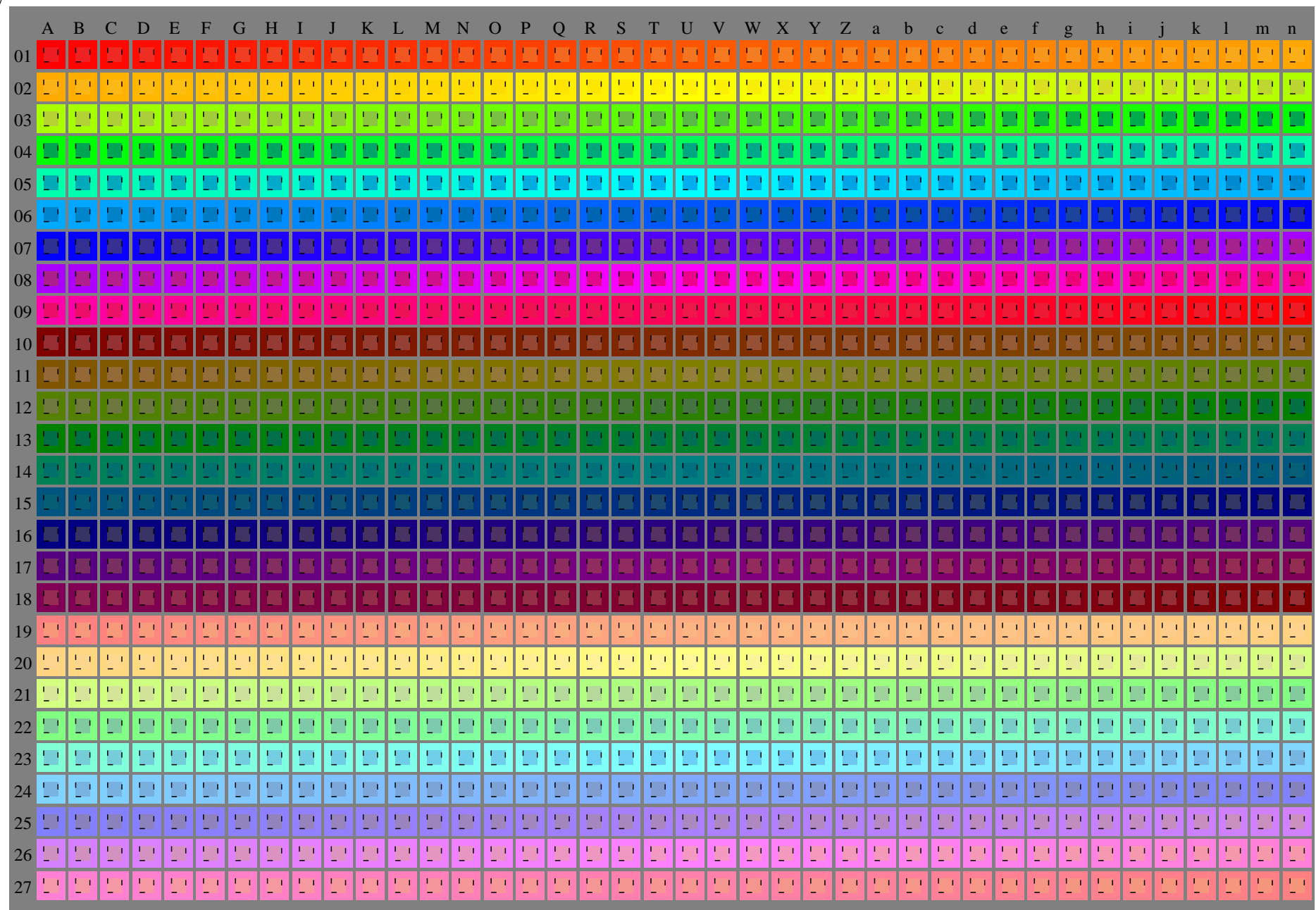
ZE810-7N, Test chart with 40x27=1080 colours; digital equidistant hue circles with 360 hues; Colour data in row 1-9, 10-18, 19-27: rgb, 245mm x 170mm. Page 1/9, ORS18
