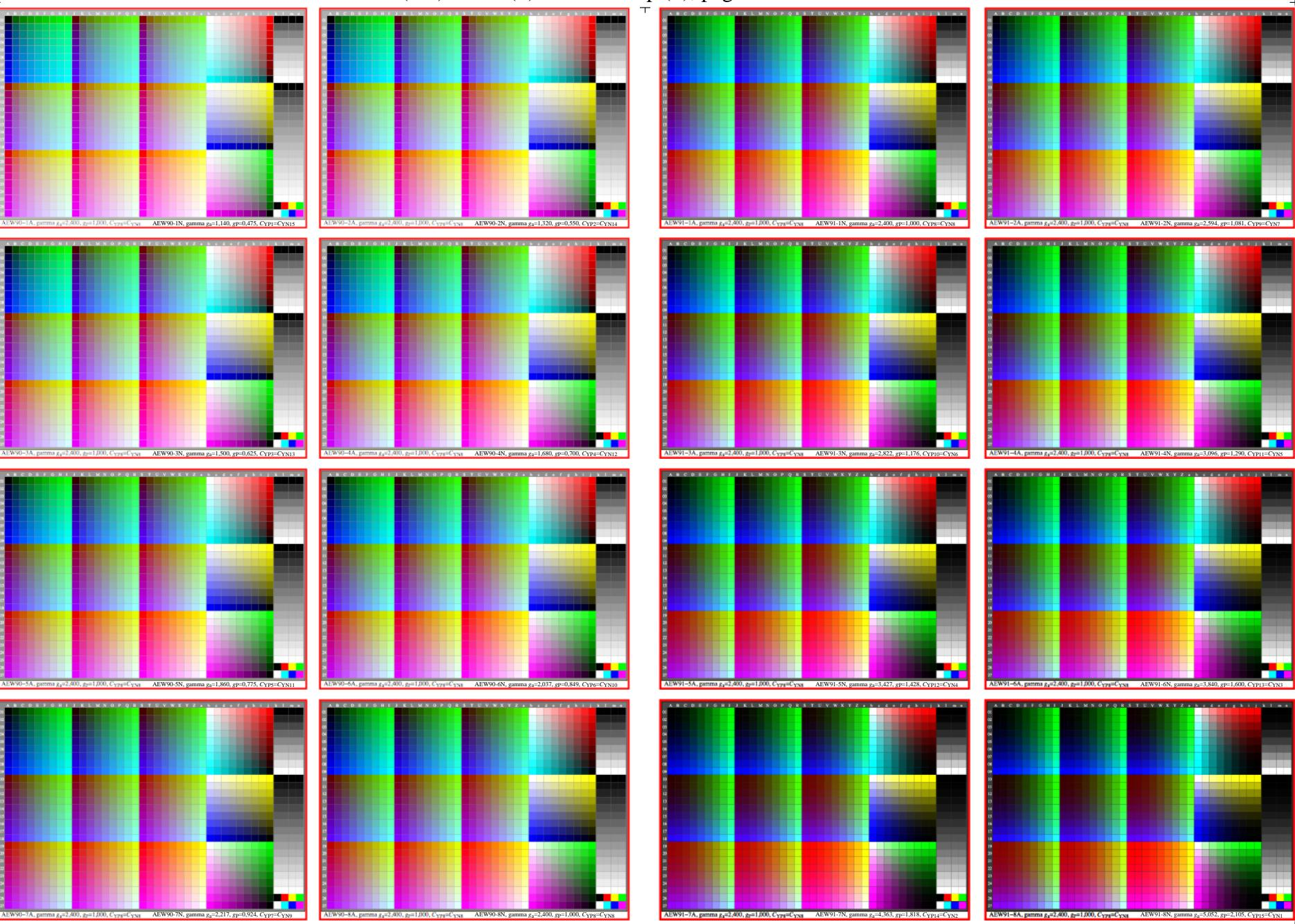
TUB-test chart AEW9; Test of optimal colour-step recognition
