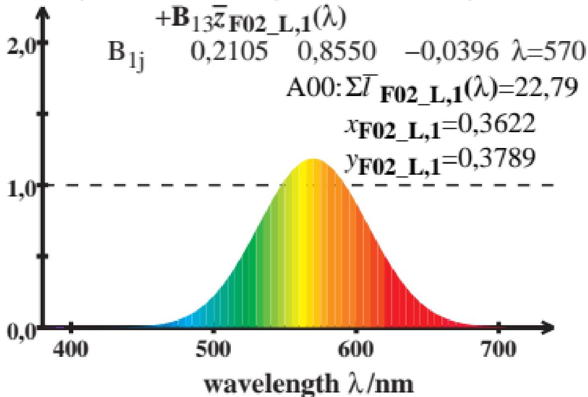
LMS\_F02\_L cone sensitivity  $\bar{y}_{\max}(\lambda)=1$
