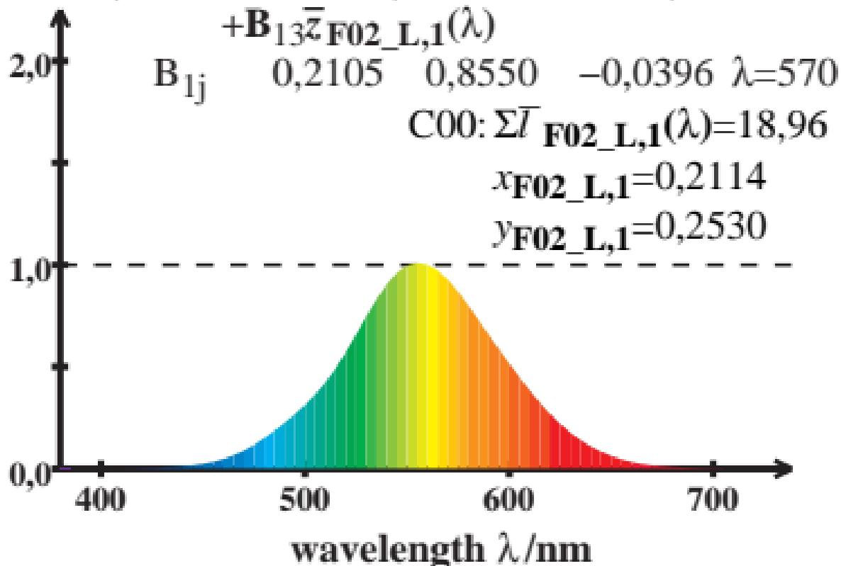
LMS\_F02\_L cone sensitivity  $\bar{y}_{\max}(\lambda)=1$
