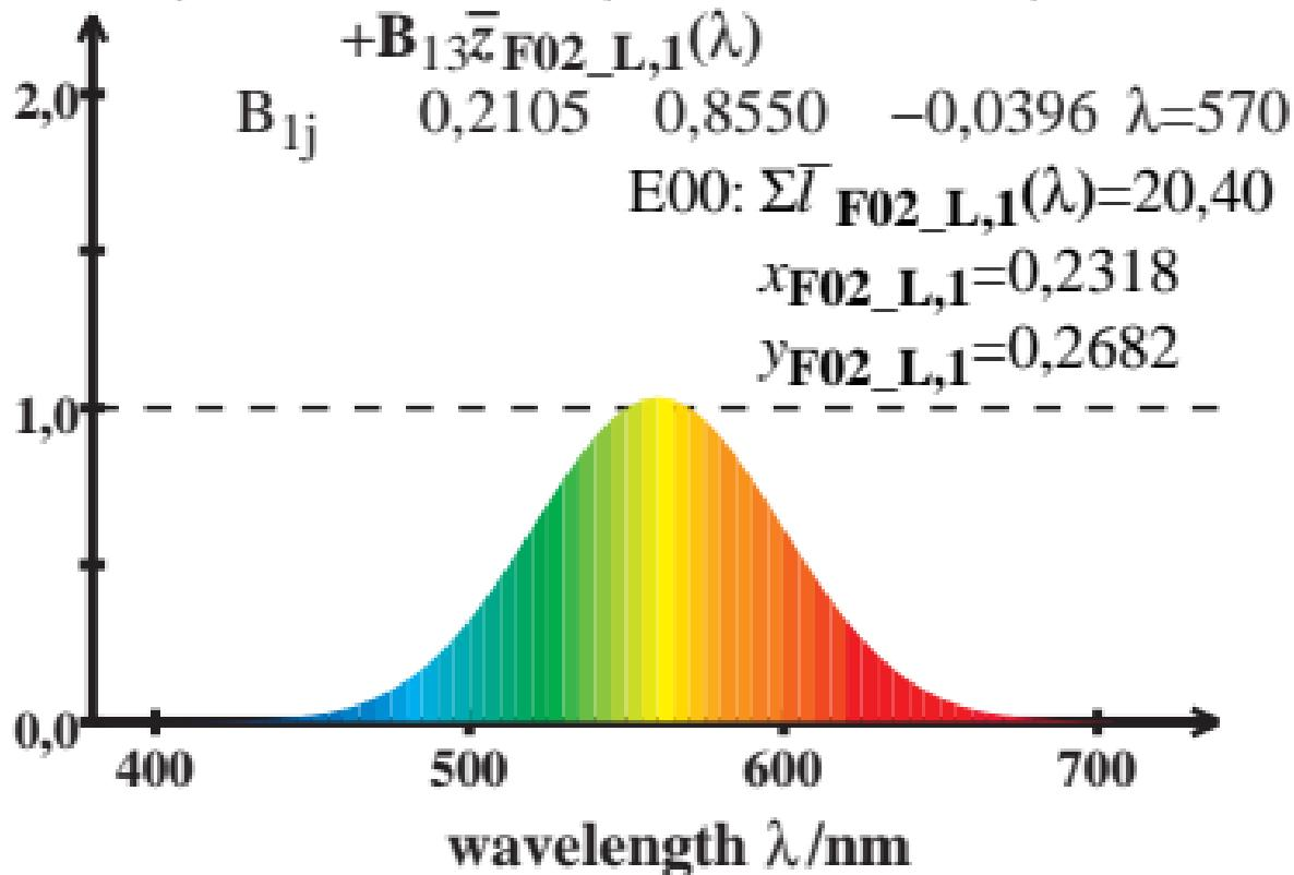
LMS\_F02\_L cone sensitivity  $\bar{y}_{\max}(\lambda)=1$
