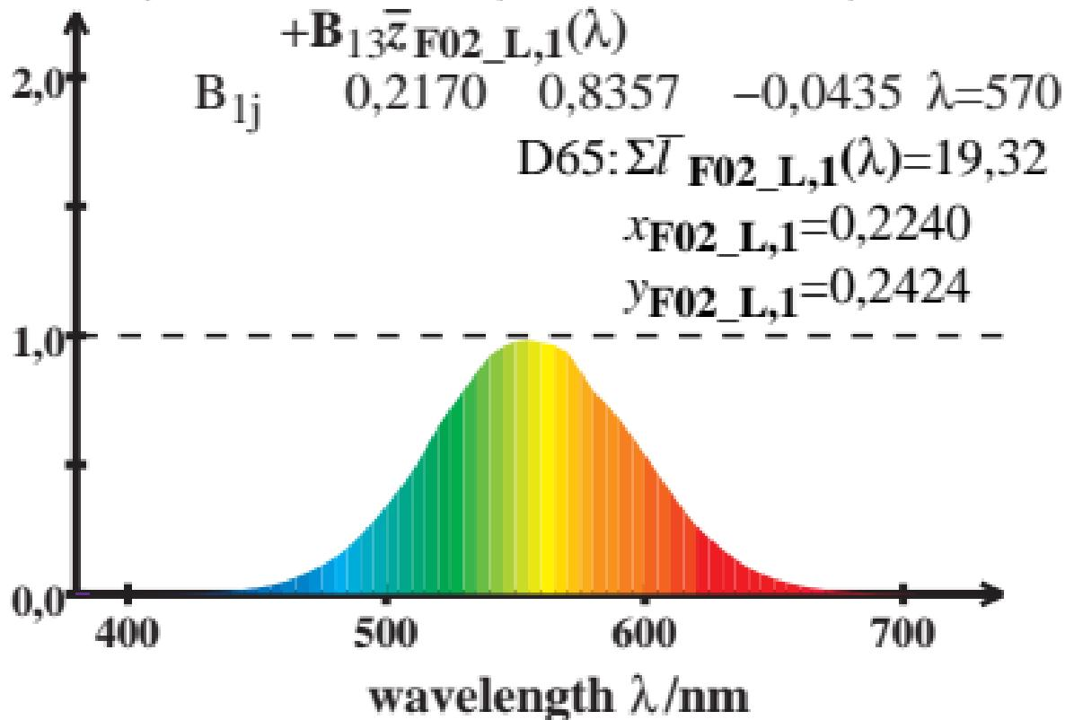
LMS\_F02\_L cone sensitivity  $\bar{y}_{\max}(\lambda)=1$
