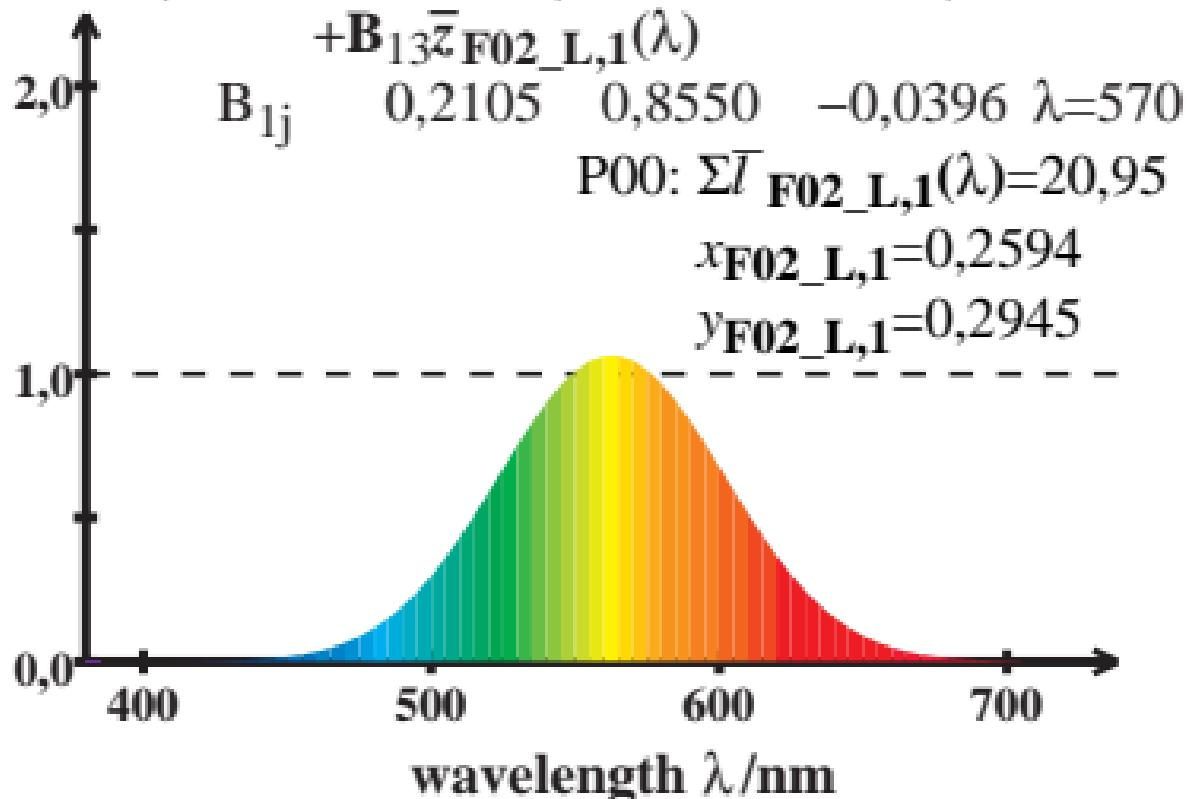
LMS\_F02\_L cone sensitivity  $\bar{y}_{\max}(\lambda)=1$
