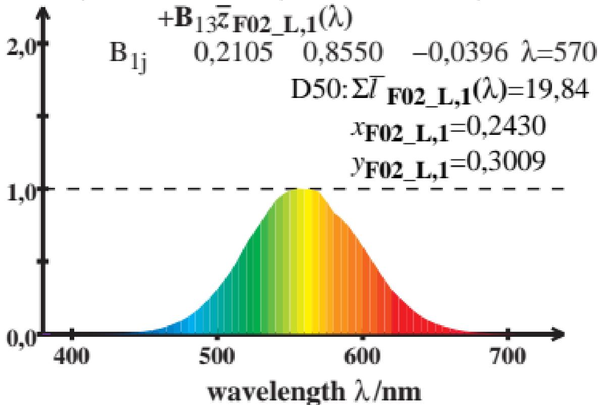
LMS\_F02\_L cone sensitivity  $\bar{y}_{\max}(\lambda)=1$
