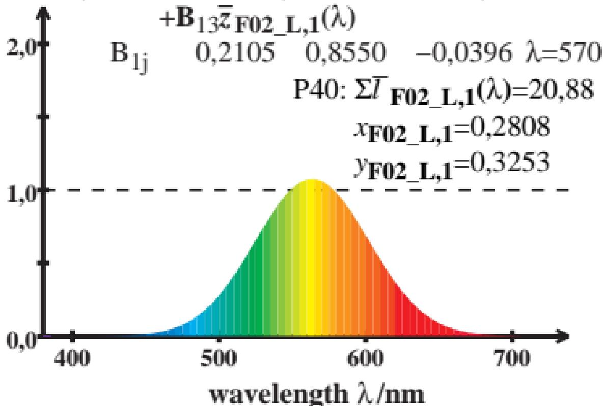
LMS\_F02\_L cone sensitivity  $\bar{y}_{\max}(\lambda)=1$
