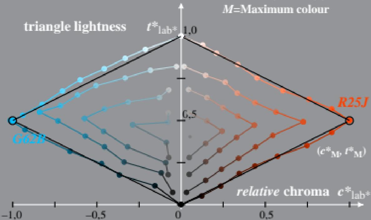
Linear relation adapted (a) CIELAB ( $C^*_{ab,a}, L^*$ ) and relative CIELAB ( $c^*, t^*$ )
