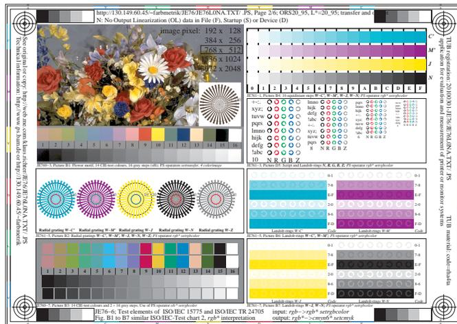
JE76-6: Test elements of ISO/IEC 15775 and ISO/IEC TR 24705
