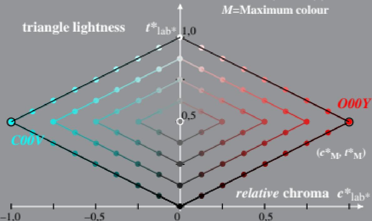
Linear relation adapted (a) CIELAB ( $C^*_{ab,a}, L^*$ ) and relative CIELAB ( $c^*, l^*$ )
