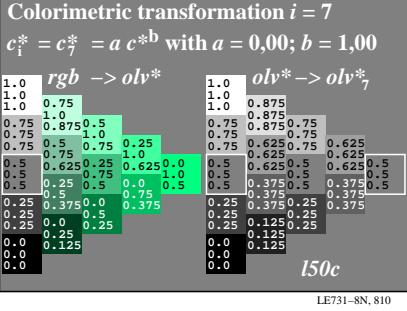
TUB-test chart LE73; Relative colour reproduction, Colour l50c input:  $rgb \rightarrow olv^*$
