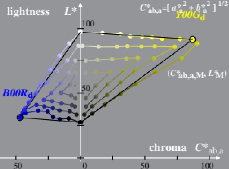
Linear relation CIELAB ( $L^*$ ,  $a^*$ ,  $b^*$ ) and adapted (a) CIELAB ( $C_{ab,a}^*$ ,  $L^*$ )
