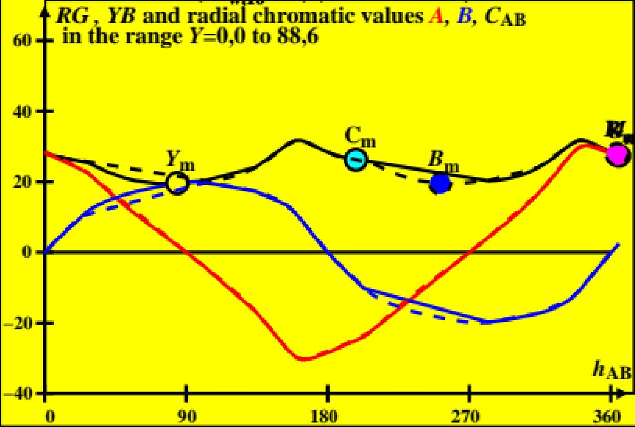
CIE data for antichromatic optimal colours of maximum chromatic value for A00,  $Y_{w,10}=88,6$ ,  $Y_m=520$  770,  $B_m=380$  520
