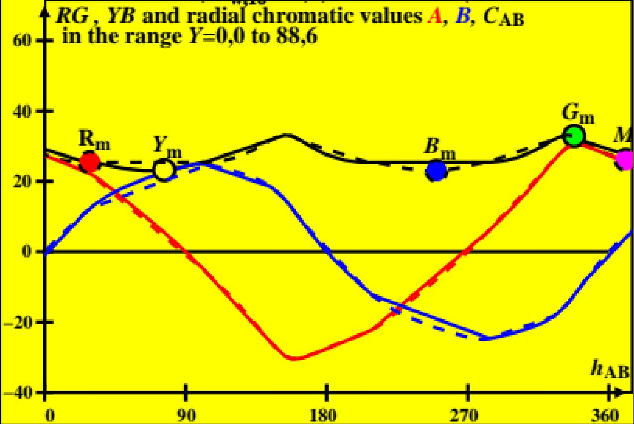
**CIE data for antichromatic optimal colours of maximum chromatic value for P40,  $Y_{w,10}=88,6$ ,  $Y_m=520$  770,  $B_m=380$  520**
