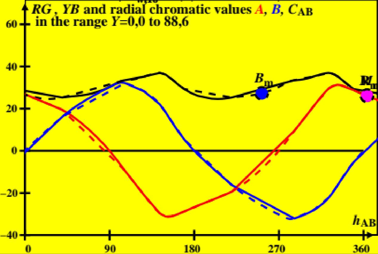
CIE data for antichromatic optimal colours of maximum chromatic value for D50,  $Y_{w,10}=88,6$ ,  $Y_m=520$  770,  $B_m=380$  520
