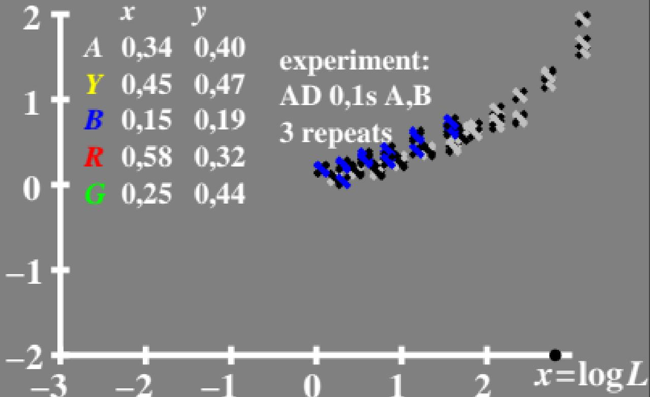
$\log \Delta L$  luminance difference threshold •  $L_g=63\text{cd/m}^2$
