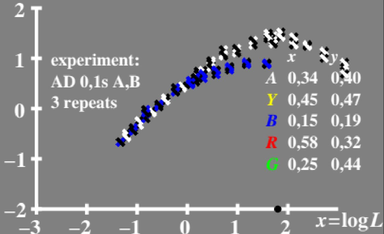
$\log L/\Delta L$  luminance contrast sensitivity threshold •  $L_g=6,3\text{cd}/\text{m}^2$
