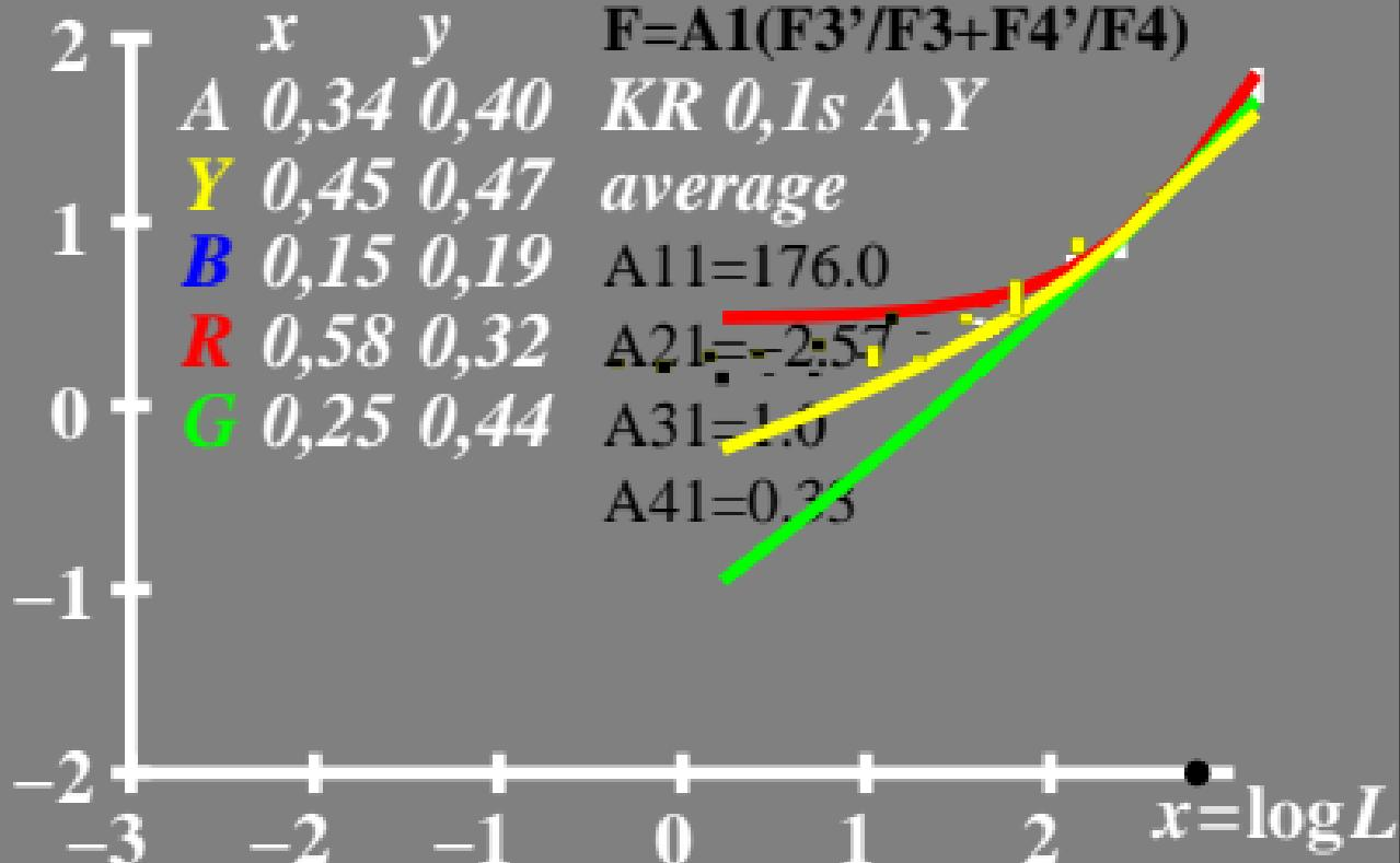
$\log \Delta L$  luminance difference threshold;  $\Delta L = L \cdot F$  •  $L_g = 63 \text{ cd/m}^2$
