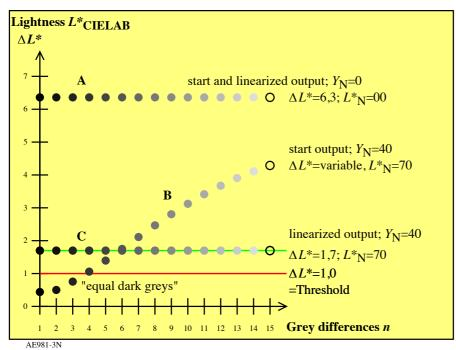
Figure 12: Lightness differences  $\Delta L^*$  of 16 grey steps for display reflections  $Y_N=0$  and 40
