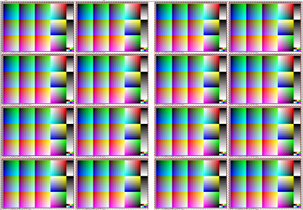
Figure 13: 16 identical ISO-test charts AE49 with the relative ISO gamma  $g_P = 0,775$  (ISO-contrast step  $C_{YP5}$ ), see <u>http://farbe.li.tu-berlin.de/AEW7/AEW70-7N.PDF</u>.
