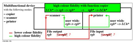
Figure 9: Multifunctional device (MFP) with three functions: copier, scanner and printer
