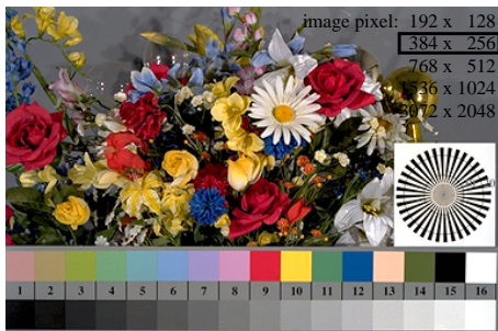
eeb80-7n, Picture D1: Flower motif, 14 CIE-test colours and 16 grey steps (nf); PS operators settransfer , 3 colorimage
