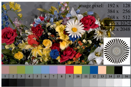
eeb81-7n, Picture D1: Flower motif, 14 CIE-test colours and 16 grey steps (nf); PS operators settransfer , 3 colorimage
