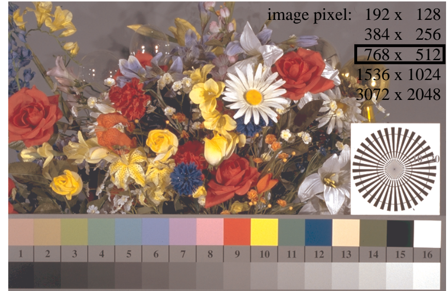
eeb91-3n, Picture B1: Flower motif, 14 CIE-test colours and 16 grey steps (sf); PS operators settransfer , 4 colorimage
