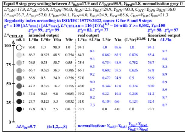
Test chart eep9; Equal 9 step grey scaling for four display reflections  $Y_{ref}=3.6, 0.4, 0.9, 1.8$ , and black  $L^*_{N,CIELAB}=17.92$ ,  $Y_N=2.5$  and white  $L^*_{W,CIELAB}=95.99$ ,  $Y_W=90$ , normalisation: grey U
