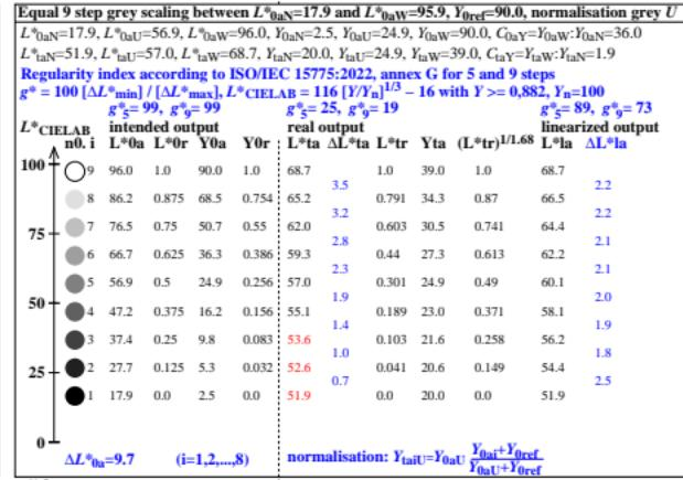
Test chart eeq9; Equal 9 step grey scaling for four display reflections  $Y_{ref}=2.5, 10, 20, 90$ , and black  $L^*_{N,CIELAB}=17.92$ ,  $Y_N=2.5$  and white  $L^*_{W,CIELAB}=95.99$ ,  $Y_W=90$ , normalisation: grey U
