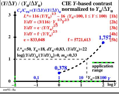
TUB-test chart eer9; Calculated for the LABJND colour-difference formula, see CIE 230:2019
