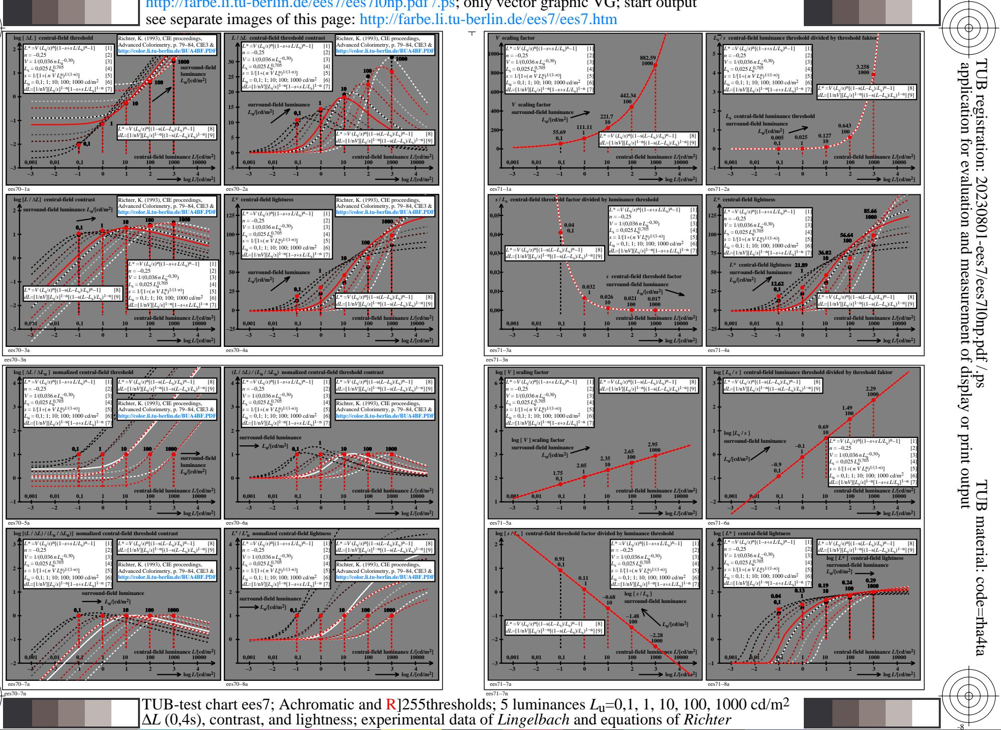
TUB-test chart ees7; Achromatic and R|255 thresholds; 5 luminances  $L_u=0, 1, 10, 100, 1000$  cd/m<sup>2</sup>;  $\Delta L$  (0,4s), contrast, and lightness; experimental data of *Lingelbach* and equations of *Richter*
