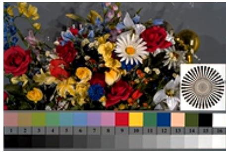
egc71-4n, eeb61-7a, ANC41-6N; nf; +2,0 stop, 192 x 128 pixel, gamma = 1,29
