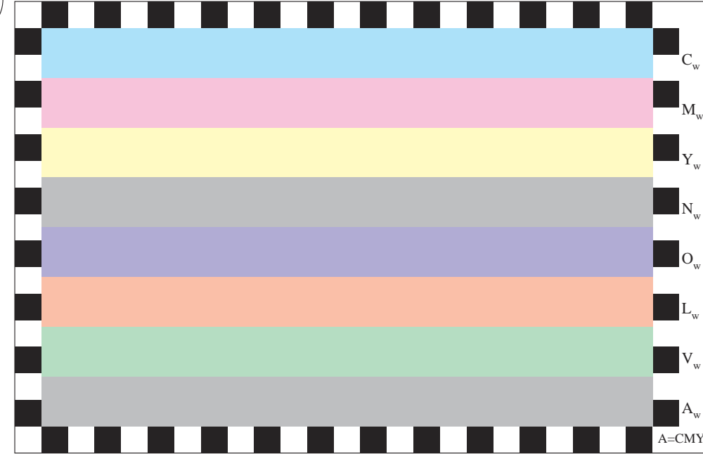
Picture D1: Colours CMYNOLVA w for homogeneity and gost images; PS operator cmly0*/000n* setcmlycolor
