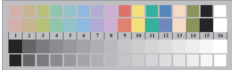
Picture B3: 14 CIE-test colours and 2 + 16 grey steps; Use of PS operator cm\dot{y}0^*/000n^* setcmykcolor
