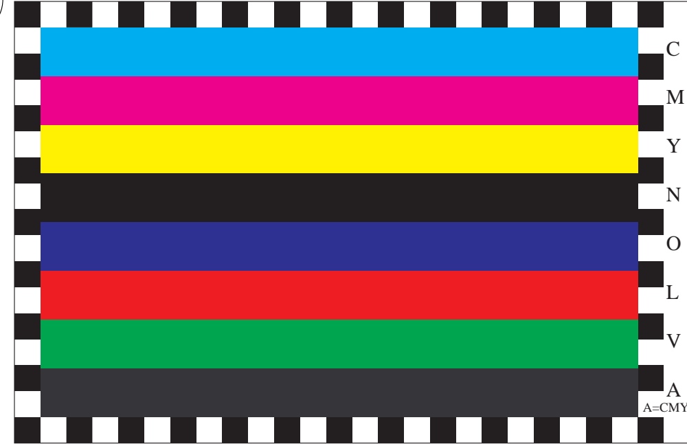
Picture B1: Colours CMYKOLVA for homogeneity and gost images; PS operator cmy0*/000n* setcmykcolor
