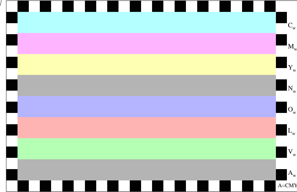
Picture D1: Colours CMYNOLVA w for homogeneity and gost images; PS operator cmly0*/000n* setcmkcolor
