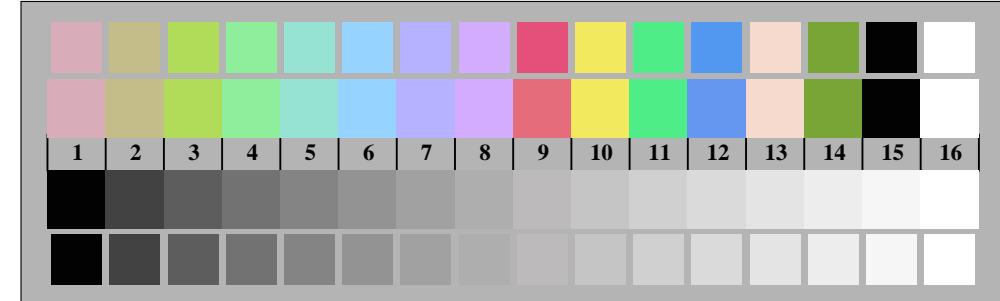
Picture D3: 14 CIE-test colours and 2 + 16 grey steps; Use of PS operator cmly0* setcmkcolor (only)
