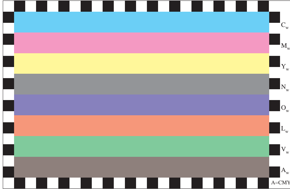
Picture D1: Colours CMYNOLVA w for homogeneity and ghost images; PS operator cmY0*/1000n* setcmYcolor (only)
