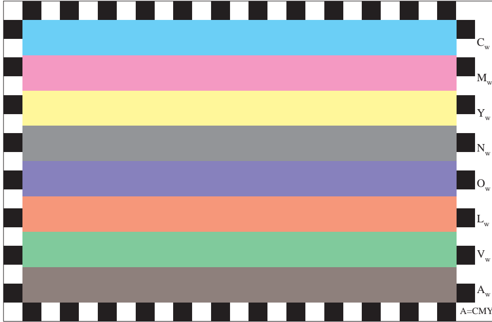
Picture D1: Colours CMYNOLVA w for homogeneity and gost images; PS operator cmY0*/000n* setcmykcolor
