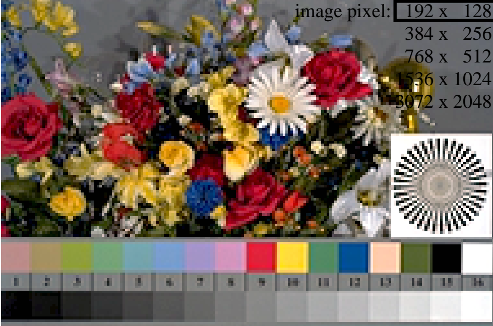
Picture D4: 16 equidistant steps W-O, W-L, W-V and W-N; Use of PS operator LAB* setcolor
