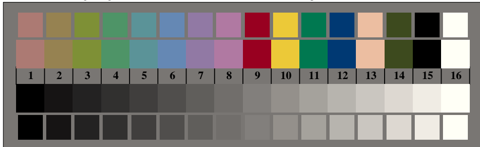
Picture B3: 14 CIE-test colours and 2 + 16 grey steps; Use of PS operator LAB* setcolor
