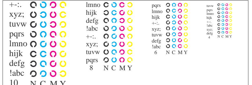
Picture B5: Script and Landolt-rings N, M, C and Y; Use of PS operator cmy0*/000n* setcmycolor
