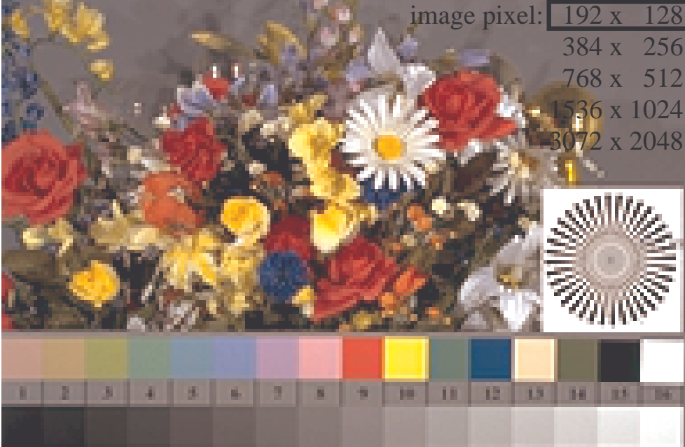
Picture B1: Flower motif, 14 CIE-test colours and 2 + 16 grey steps (sf); PS operators settransfer , 4 colorimage
