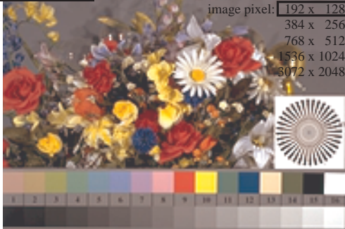
Picture B1: Flower motif, 14 CIE-test colours and 2 + 16 grey steps (s); PS operators settransfer , 4 colorimage
