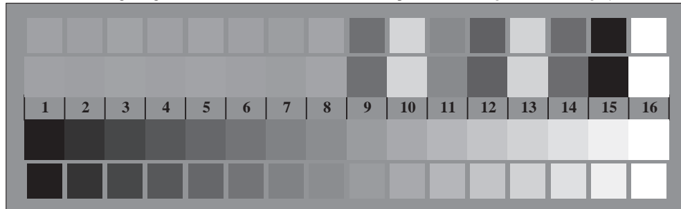
Picture B3: 14 CIE-test colours and 2 + 16 grey steps; Use of PS operator olv* setrgbcolor / w* setgray
