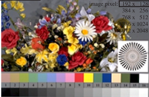
Picture B1: Flower motif, 14 CIE-test colours and 2 + 16 grey steps (s); PS operators settransfer , 3 colorimage
