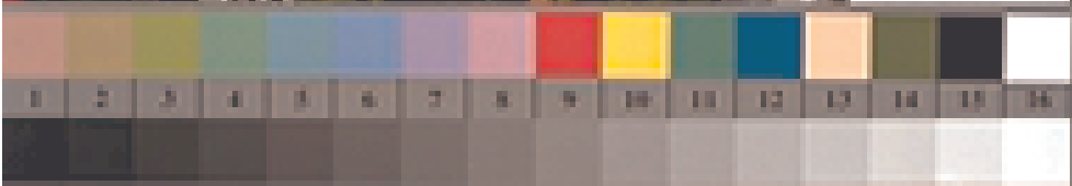
Picture D1: Flower motif, 14 CIE-test colours and 2 + 16 grey steps (nf); PS operators settransfer , 4 colorimage
