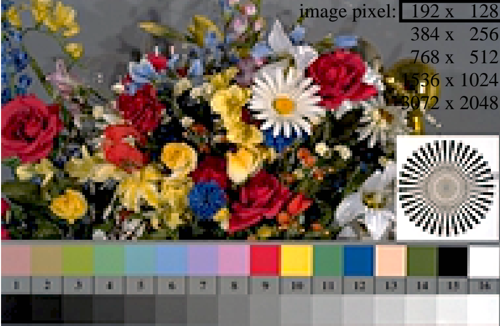
Picture D1: Flower motif, 14 CIE-test colours and 2 + 16 grey steps (nf); PS operators settransfer , 3 colorimage
