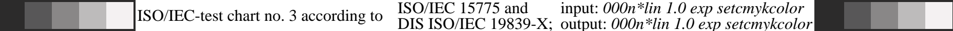
Picture C3: 16 visual equidistant L^* -grey steps; PS operator: 000n* setcmykcolor; use file www.bam.de/FE86/10L/L86E0iNA.PS or L86E0iNP.PS .PDF (i=0,7) for PDF systems to complete the figure
