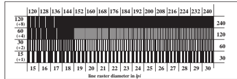
Picture C6: Line raster under 90° (or 0°); Use of the PS operator 000n* setcmykcolor
