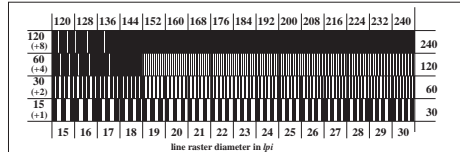
Picture C6: Line raster under 90° (or 0°); Use of the PS operator w w w^* \text{setrgbcolor}
