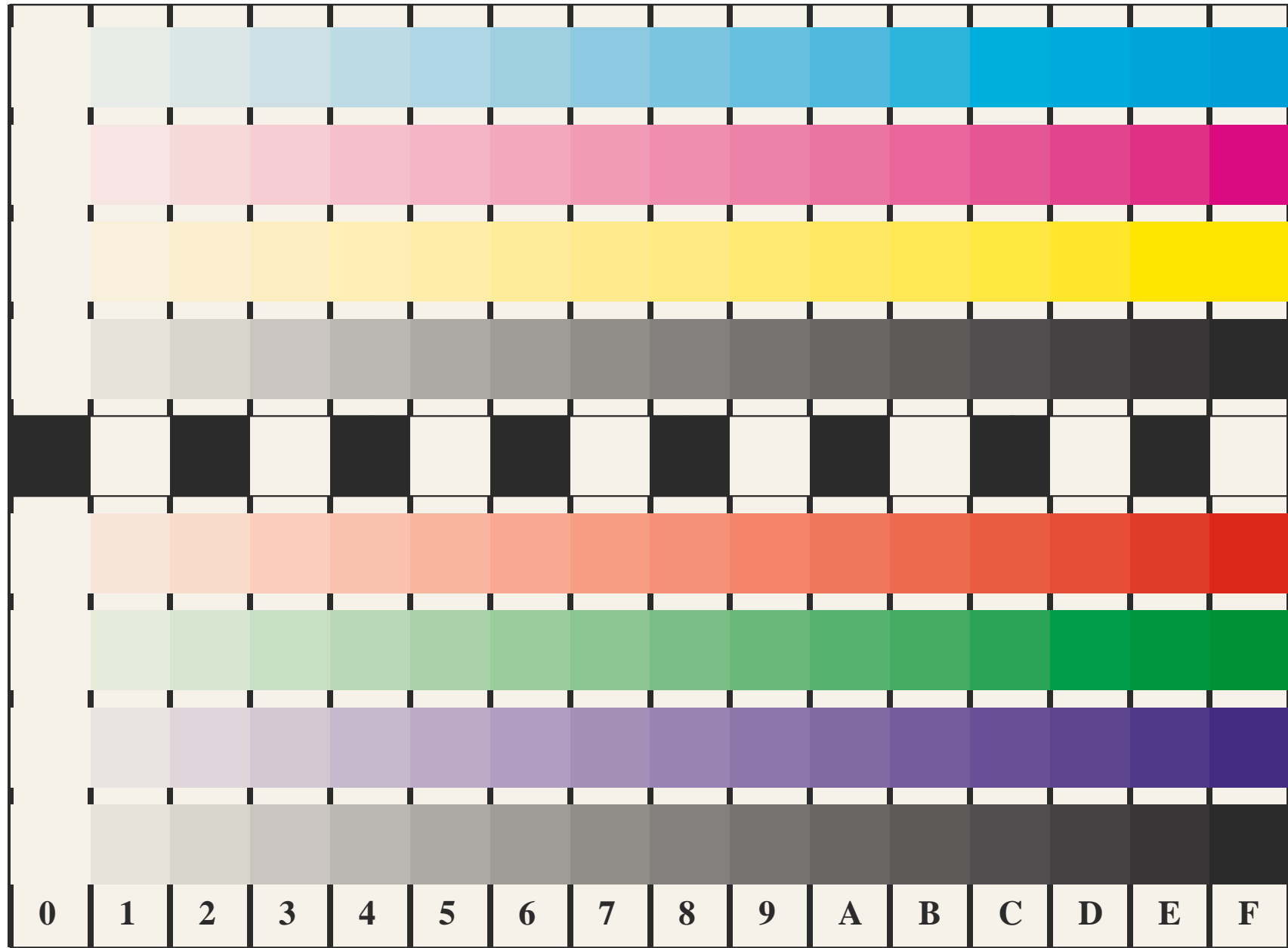
Picture B4 and D4: 16 equidistant steps B4 : W-C, W-M, W-Y and W-N; D4 : W-O, W-L, W-V and W-N(CMY); Use of PS operator; B4: olv* setrgbcolor / w* setgray; D4: olv* setrgbcolor (only)
