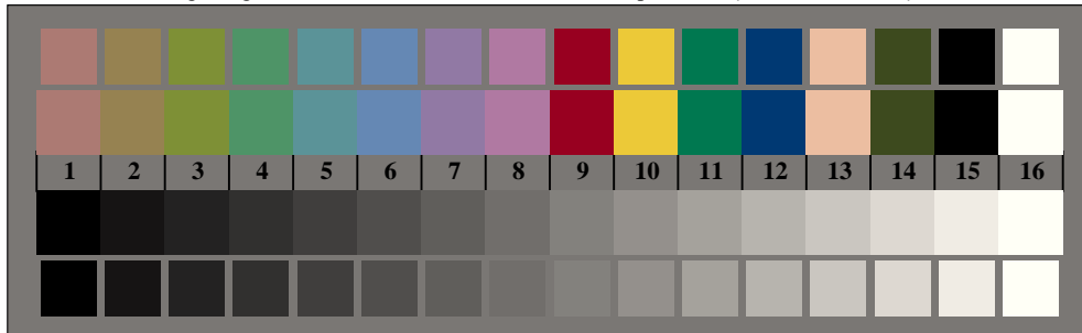
Picture B3: 14 CIE-test colours and 2 + 16 grey steps; Use of PS operator cmly0*/000n* setcmlycolor
